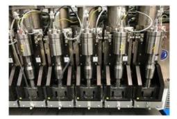
A booster and the sonotrodes are used to apply the mechanical oscillations generated from electrical signals to the web being bonded.
