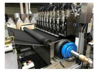
In the ultrasonic welding plant, two layers of nonwovens and one vapor-permeable film are merged with one another in a continuous lamination process to create roofing underlays.
