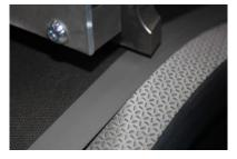
The high productivity and cost efficiency of the process were the key motivation behind the decision to go with ultrasonic welding. All of the company's products, regardless of their thickness, can be laminated effectively and accurately using the system.
